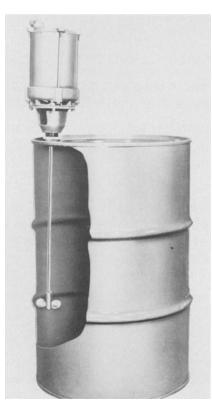
MIXERS FIT 55-GALLON DRUMS Bung mixers, designed with a specially threaded connection to screw into standard 55-gallon drums, are being marketed by Neptune Mixer Co. The Series E bung mixers are vertically mounted and feature folding blades for easy drum entry, says the company. In operation, the blades open up to 3-3/4-in. for mixing. The mixers can be supplied with air or electric motors. Contact: Mike Dowse, vicepresident, Neptune Mixer Co., PO Box 247, Lansdale, PA 19446.
